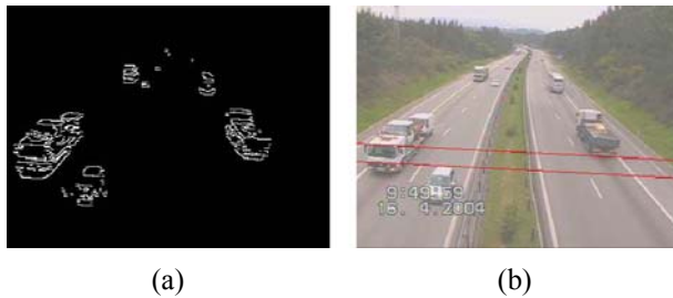
Fig. 2. (a) Edges detected by applying the Sobel Detector to the segmented vehicles. (b) Lines identified using the edges represented in (a) are outliers, the estimation of this vanishing point using the least squares method is ill-conditioned.
