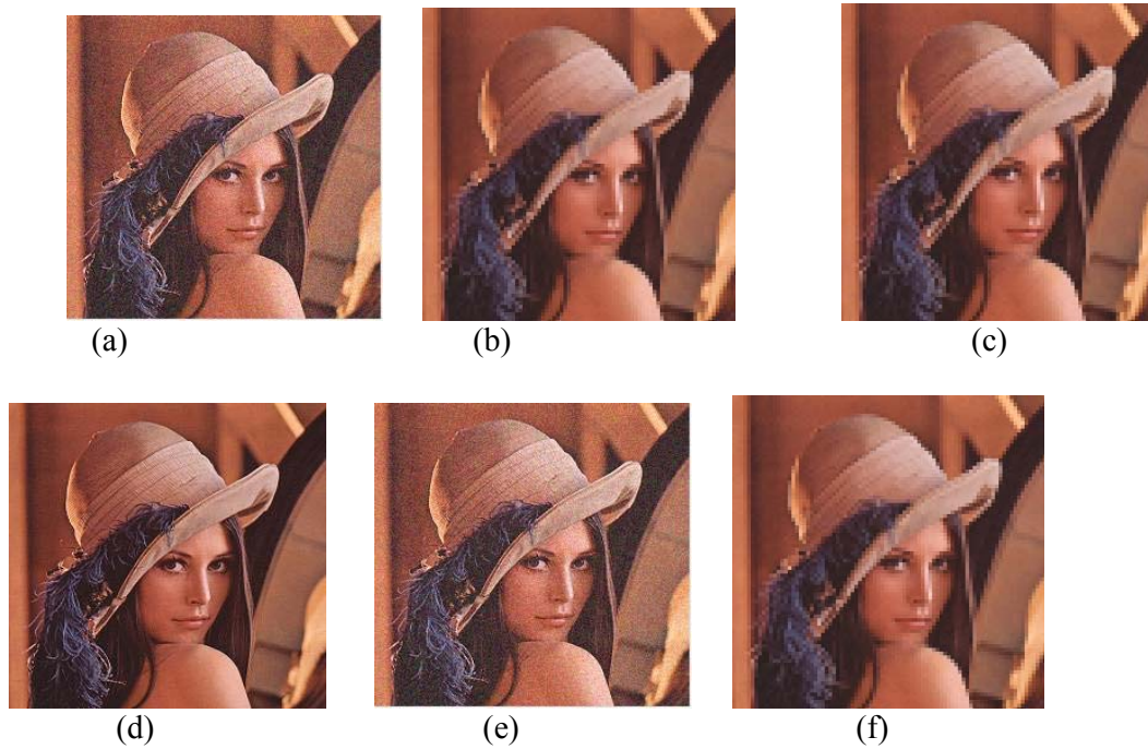
Figure 2. Restoration of Lena image. (a) Original image, (b) Corrupted image with Gaussian noise \sigma=15 , (c) recovered image by median filter, (d) recovered image by mean filter, (e) recovered image with vector median filter, and (f) is the result of recovering image by proposed fuzzy filter.
