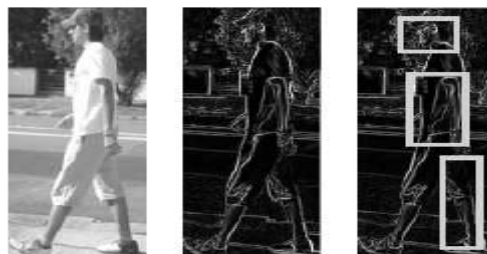
Fig 3:Left: an image window. Middle: the edge magnitude. Right: three edge density features
