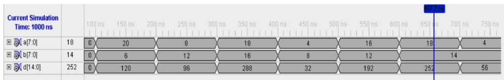
Fig. 2. Simulation results of Karatsuba algorithm using polynomial multiplication
