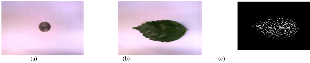
Figure 3: (a) Coin image used as reference (b) Hibiscus leaf image (c) Edge image of Hibiscus leaf
