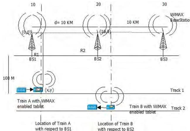
Figure 2. Representation of train's running on same track and in opposite direction
