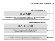
Fig 1: Extensibility of IEEE 802.11s with respect to path selection protocols [25]
