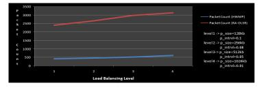
Fig 4: Packet count of HWMP and RA-OLSR for different values of packet size and packet interval.
