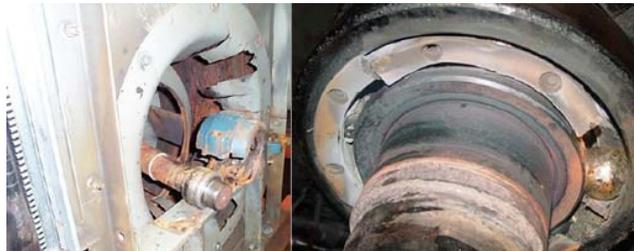
Fig. 1 Damage Observed In Machines Due To Uncontrolled Vibrations
