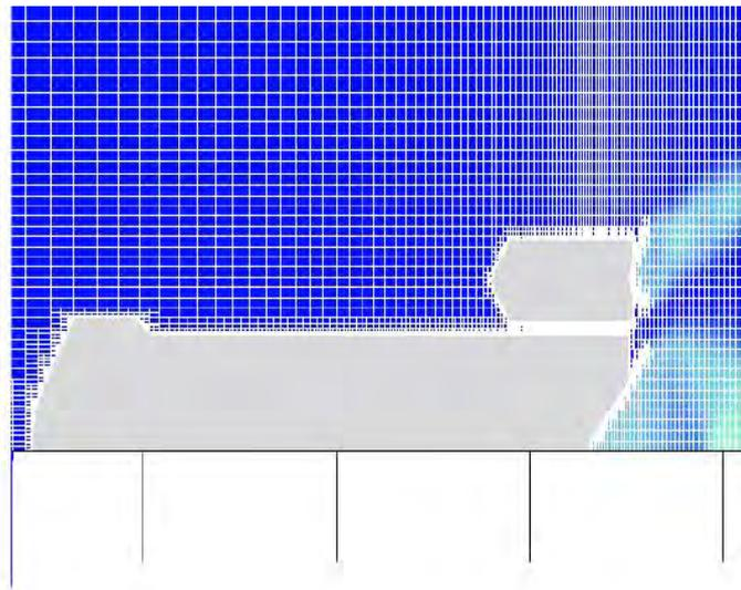
Figure.1 Blown-up view of grid distribution .
