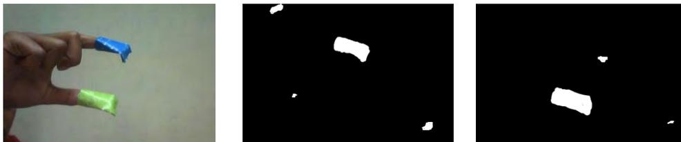
Fig. 1. (L to R) The input frame, thresholded image for blue, thresholded image for green
