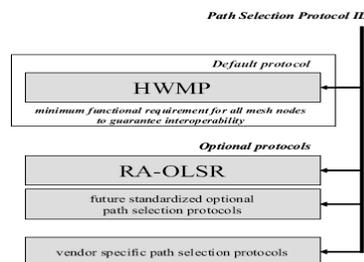
Fig 1: Extensibility of IEEE 802.11s with respect to path selection protocols [25]
