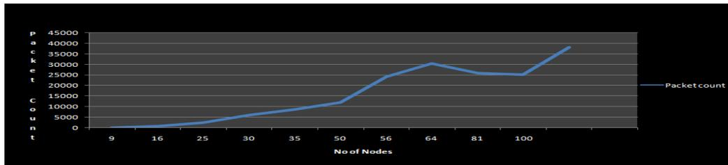
Fig 3: Packet counts at different number of nodes using RA-OLSR
